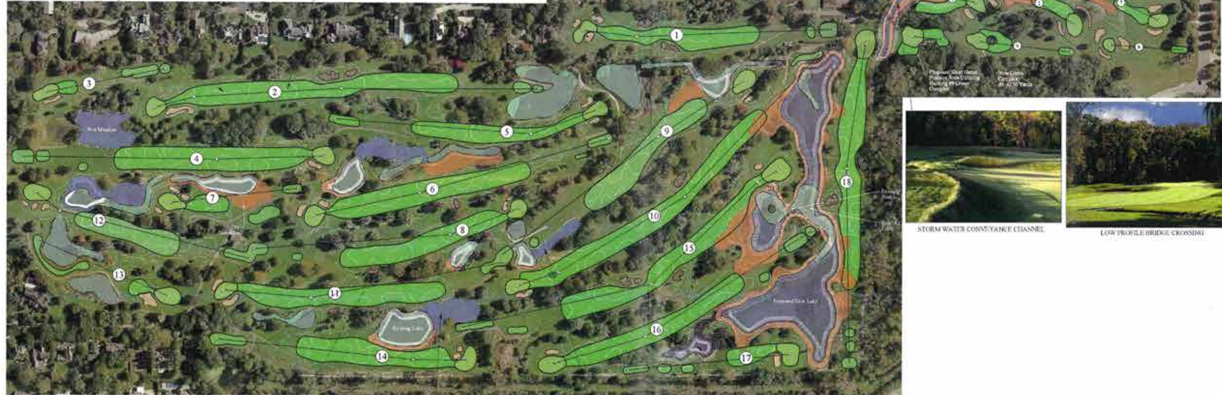
AFTER ENHANCED SURFACE SLOPE PROVIDES ADEQUATE SURFACE DRAINAGE TO PROPOSED DRAINAGE INLETS
