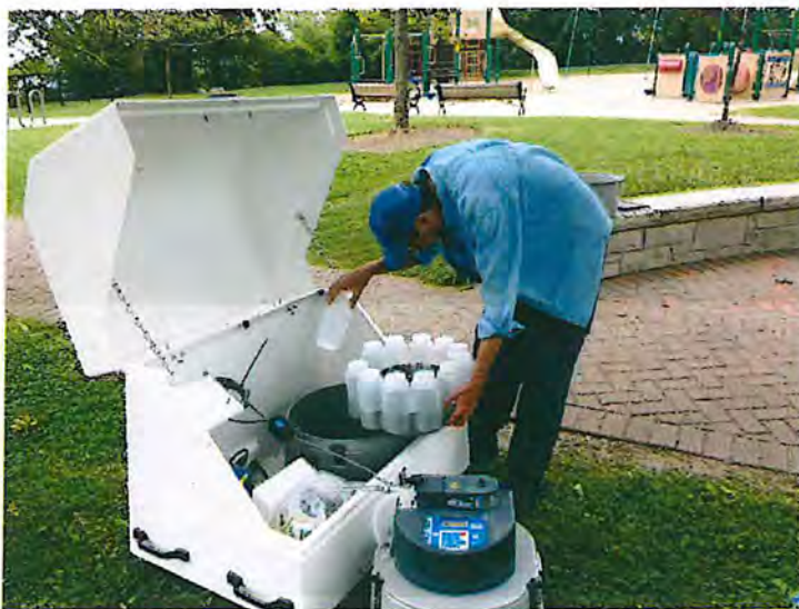
Installation within fiberglass enclosure. Rain gauge mounted on 4x4 post.
