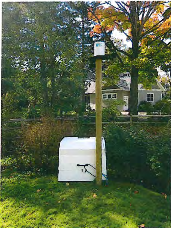
Installation within fiberglass enclosure. Rain gauge mounted on 4x4 post.
