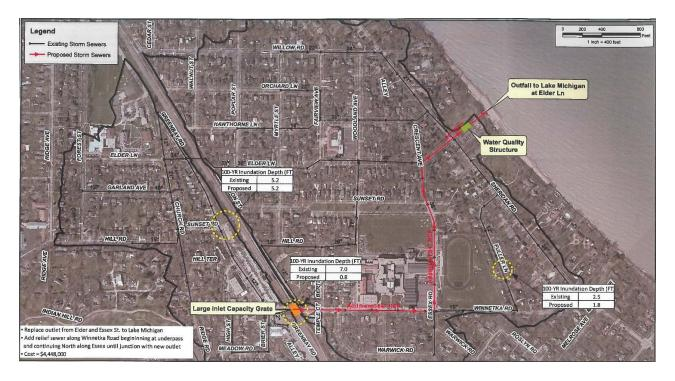
The watershed area is the largest Lake Michigan watershed in east Winnetka, and the only east side watershed that also includes areas west of the railroad tracks as the system crosses under the UP-N tracks to the Elder outfall. There are two existing outlet pipes at the Elder outfall, a 24-inch and 27-inch pipe. This stormwater conveyance system has been in place since the 1940's when the railroad tracks were lowered.
