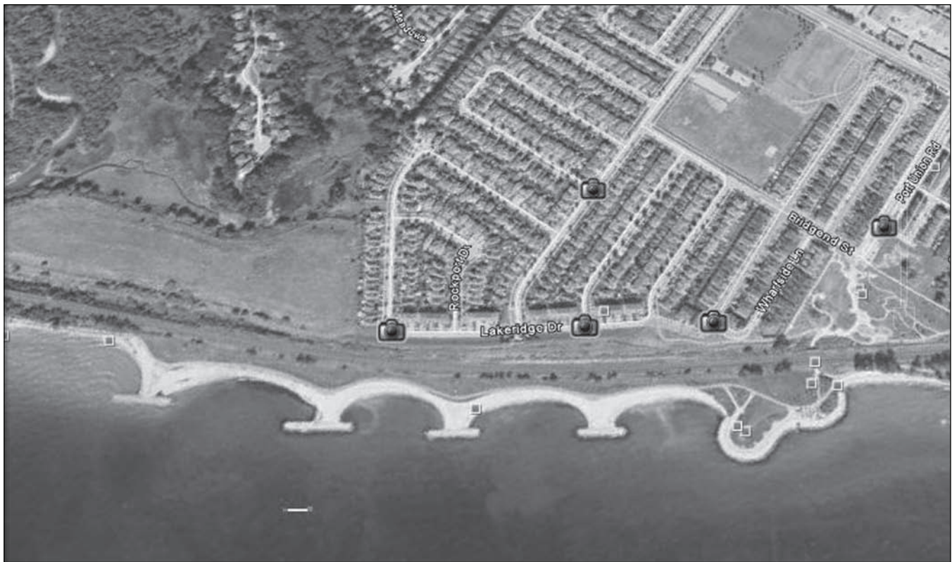
Figure 6. Armored headland and attached breakwaters constructed in 2005-2006 to protect public beaches in Port Union, Ontario. A second system was constructed about a half mile to the north in 2009. Note 100-ft scale bar (Google air photo 2009).
