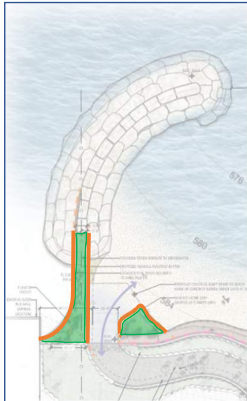
North planting pocket (planting pocket shown in green, steel shown in orange)
